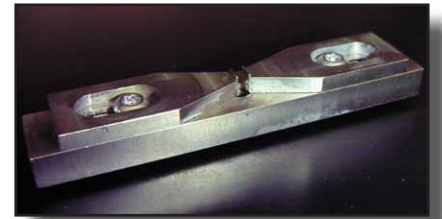
Figure 2 - Bottom span of custom 4-point bend fixture.
