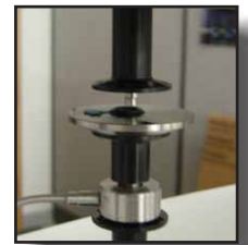
Figure 1 - Monolayer of microspheres prior to test
